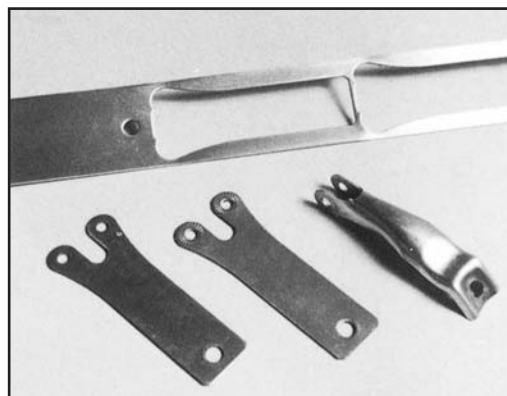
Stainless steel fastener blanked with an ASP 23 die and VANADIS 4 punch.
